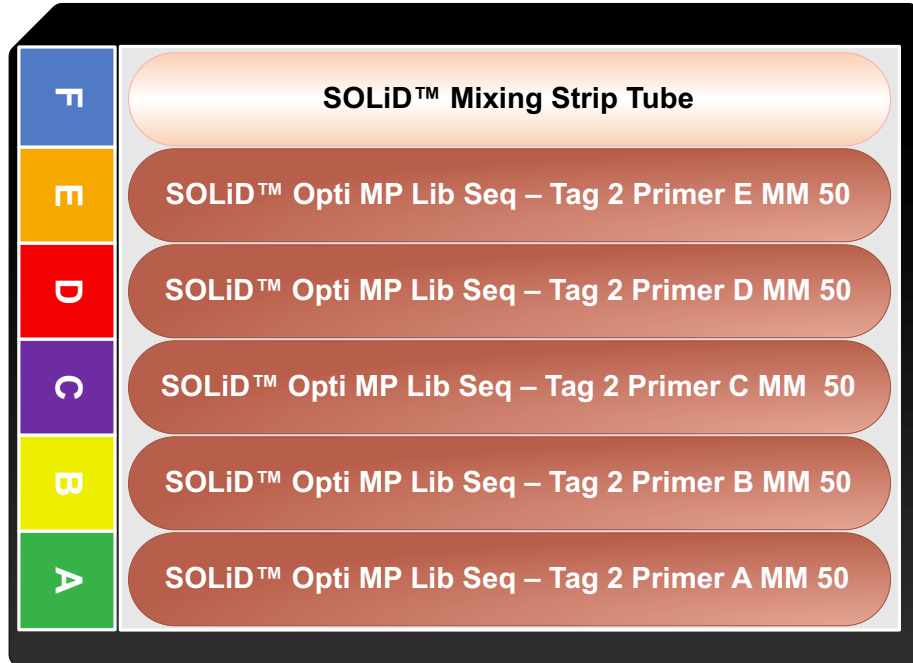
Figure 29 Reagent strip block layout to sequence mate-paired Tag 2 (50 bp).
