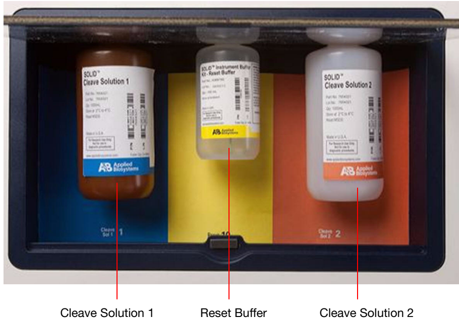
Figure 15 Positions of reagent bottles on the side of the instrument.
