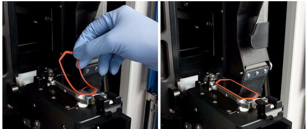
Figure 74 Install the SOLiD™ O-Ring on a flowcell.
