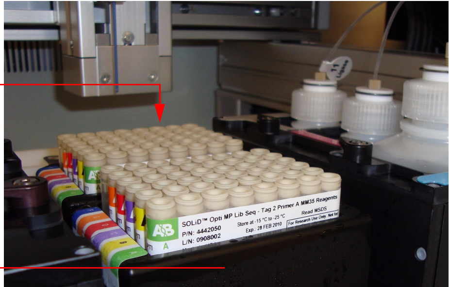
Figure 34 Position of the sequencing reagent blocks for flowcells 1 and 2.
