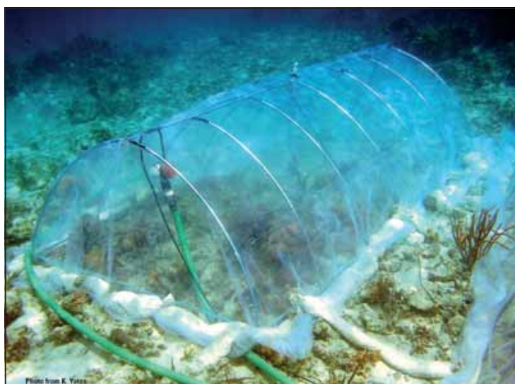
Figure 13.4 Underwater enclosure (SHARQ) deployed in the U.S. Virgin Islands. The SHARQ is used for in situ perturbation studies on the impact of ocean acidification on benthic communities (photo credit: K. Yates).
